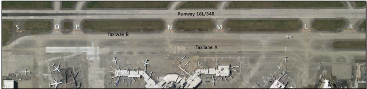
Figure 2-10 Connector Taxiways with Direct Access to a Runway from an Apron Seattle-Tacoma International Airport
